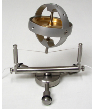
Figure 5.12: Why a fast-spinning gyroscope seems to balance much more easily on a stretched spring than a non-rotating body?
