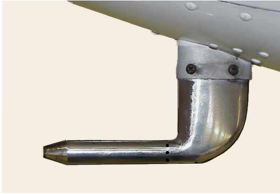
Figure 6.13: A Pitot tube and the principle of its operation
