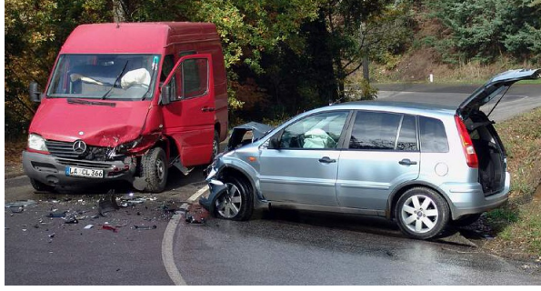
Figure 5.7: The result of a car crash. The delivery van has stopped almost on the spot in its original track, but the passenger car, which, before the crash had been traveling along the solid line, has ricocheted, and it has been turned around by approx. 90^\circ . Luckily, nobody was seriously injured.
