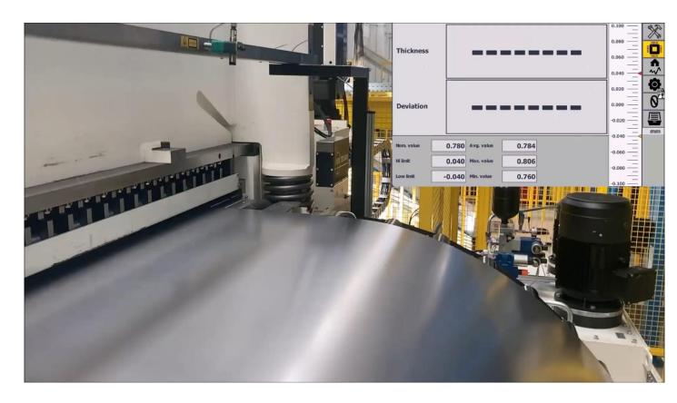
Inline Monitoring of Coil Quality in Controlled Punching and Forming Processes
